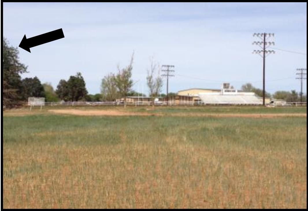
View to the northwest of the mark set for the tower location. The arrow points to the end of the windbreak that will have to be trimmed to allow clearance for the tower's northwest guywire. It's estimated that 5-8 trees be removed from this area to allow a free path for the line. The entire field was recently planted by the ISD with oat grass to keep the soil in place and blowing dust in check.
