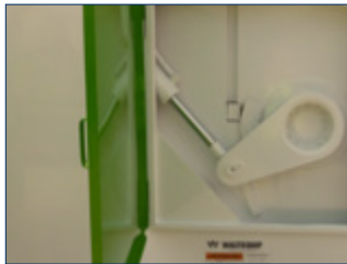
Easily accessible shielded hydraulic cylinders and hoses
